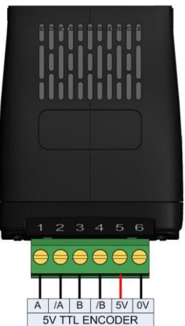
Connection Example – 5V TTL Encoder OPT-2-ENCOD-IN
