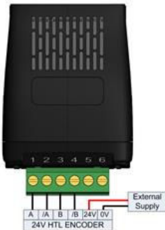
Connection Example – 24V HTL Encoder OPT-2-ENCHT-IN
