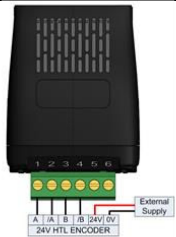
Connection Example – 24V HTL Encoder OPT-2-ENCHT-IN
